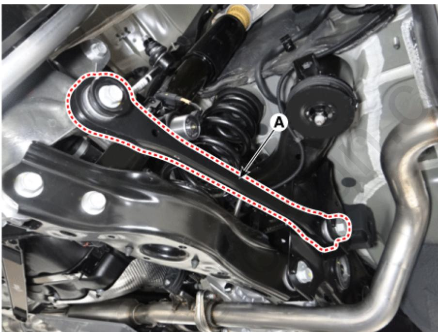
6. Loosen the rear lower arm bolt & nut and then separate the lower arm from the rear axle.
