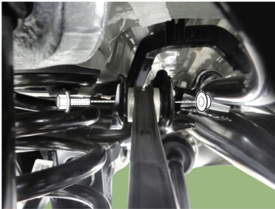
11. Loosen the bolt & nut and then remove the rear upper arm front from the rear axle.
